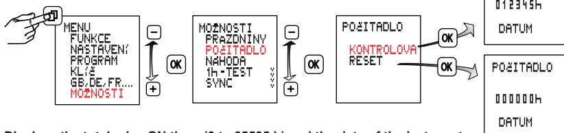
Displays the total relay ON time, (0 to 65535 h) and the date of the last reset.
