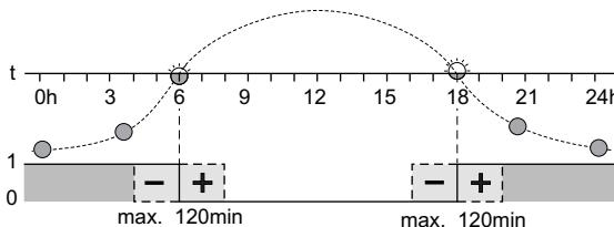
The time switch switches on at the calculated sunset time and off at the calculated sunrise time.
