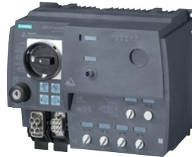
M200D AS-i Standard with manual local operation
