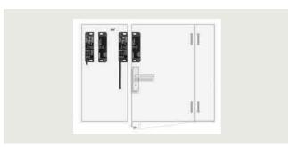
Non-contact safety magnetically operated switches (with plug or cable) for right-hinged door
