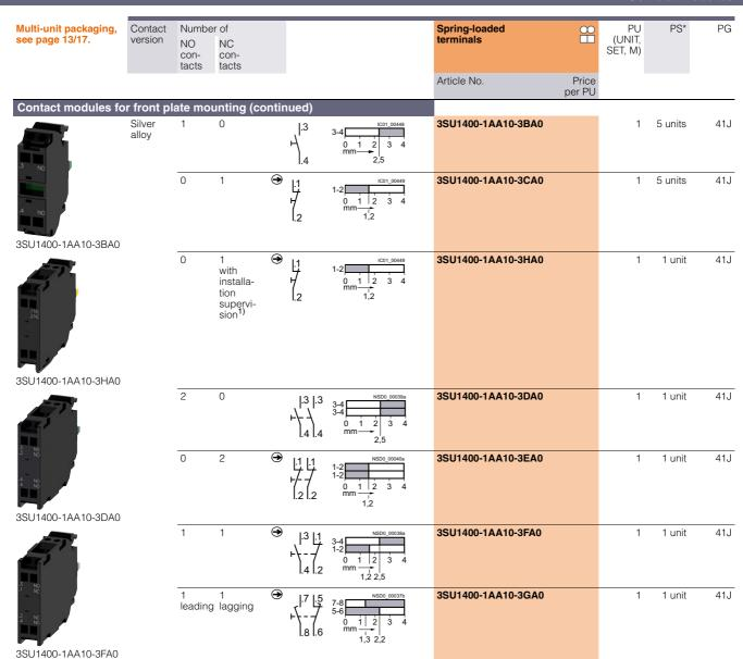
→ Positive opening according to IEC 60947-5-1, Annex K. Can be used with 3SK safety relays, see page 11/1 onwards. Certificate:
