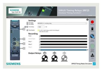
The 3RP25 simulator visualizes different time functions in the 3RP25 timing relay. Any fault scenario can be simulated.
