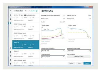
Easy input of motor and load data
