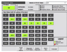
Diagnostics for AS-Interface via HMI panel
